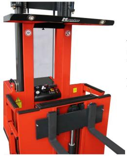
Halogen spots in the overhead guard and a fork carriage with adjustable forks are standard..
