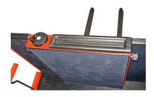
As option levers for driving, lifting and steering on both sides available. Without any change of components the driver can control the truck at both sides.
