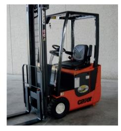
Really compact forklift 85 cm width, voltage 48 V, 2 AC traction motors, electric steering, rear twin super elastic tyres are some of the features that make the series N 08-10 the most advanced in the
